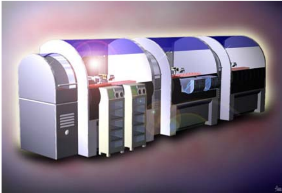
Figure 32: Modular Architecture Micro-Assembler (Courtesy of TNO Industries)
